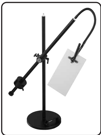
Articulated 360° clamp COGEU gives the swivel arm great, continuous mobility. Sliding weight CEGOU counterbalances even heavy loads. Safety ring CEGEE 25 , at the end of the COMBITUBE , prevents the weight from sliding off accidentally.
