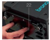
springs in the battery compartment are not dirty or damaged. When changing the battery press the locking mechanism at the bottom (22) together using finger and thumb. The two big contact springs slide the battery out so far that the user may grip it.
